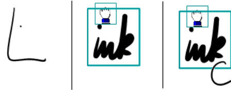
Figure 4: Left-to-right: A crop stroke is drawn indicating a paste action. The paste rectangle’s lower-left corner is aligned with the crop stroke’s corner. The pasted selection is copied by drawing a ‘C’ over it.
